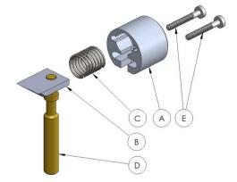
1. Begin by removing the two screws (E) to remove the cutting blade mechanism from the Peeler. Be aware that the assembly is under some spring pressure. Make a note of how the blade (B) and lever (D) fit into the cap to help during reassembly.
